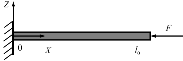
Figure 4.3 Model of a cantilever inflating beam under axial compression load.
