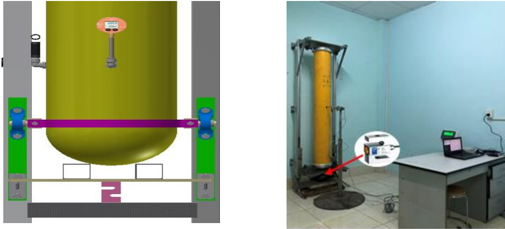
Figure 5.29 Mounting load cell type Z to the structure and restraints at top and bottom of an inflatable beam
