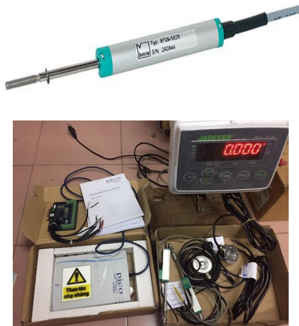
Figure 5.30 Linear Variable Differential Transformer
