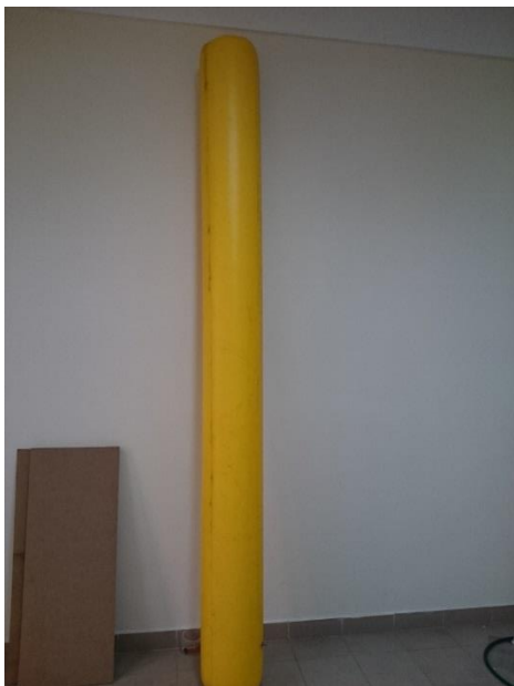
Figure 5.23 Inflatable beam after pumping
